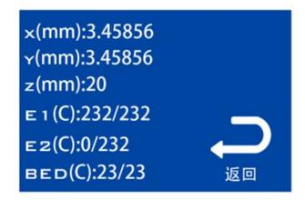
X (mm): X axis current location Y(mm): Y axis current location Z (mm): Z axis current location
